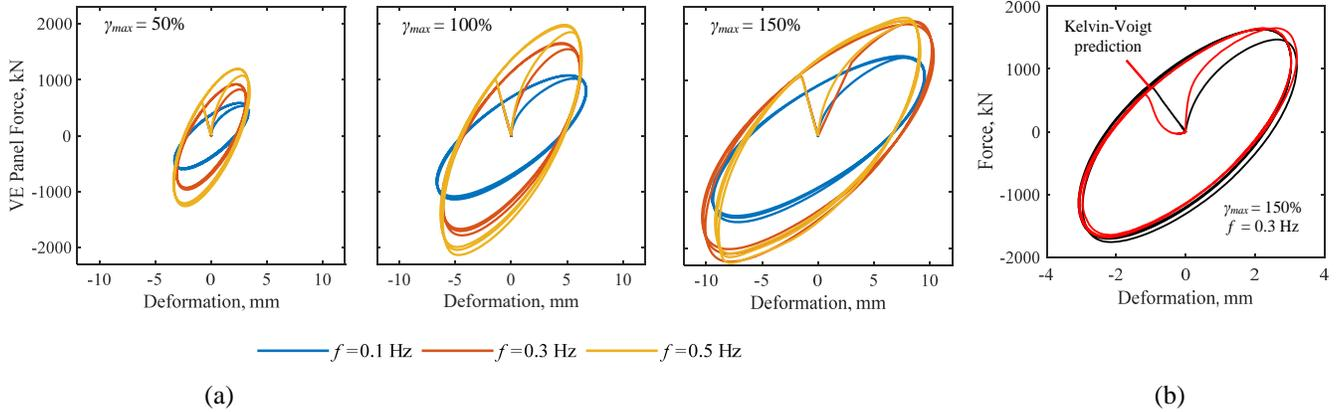
Figure 5. (a) VE Panels A hysteretic response at various frequencies and strain amplitudes (b) Harmonic tests results at  $\gamma = 150\%$  and  $f = 0.3$  Hz and comparison with Kelvin-Voigt model.
