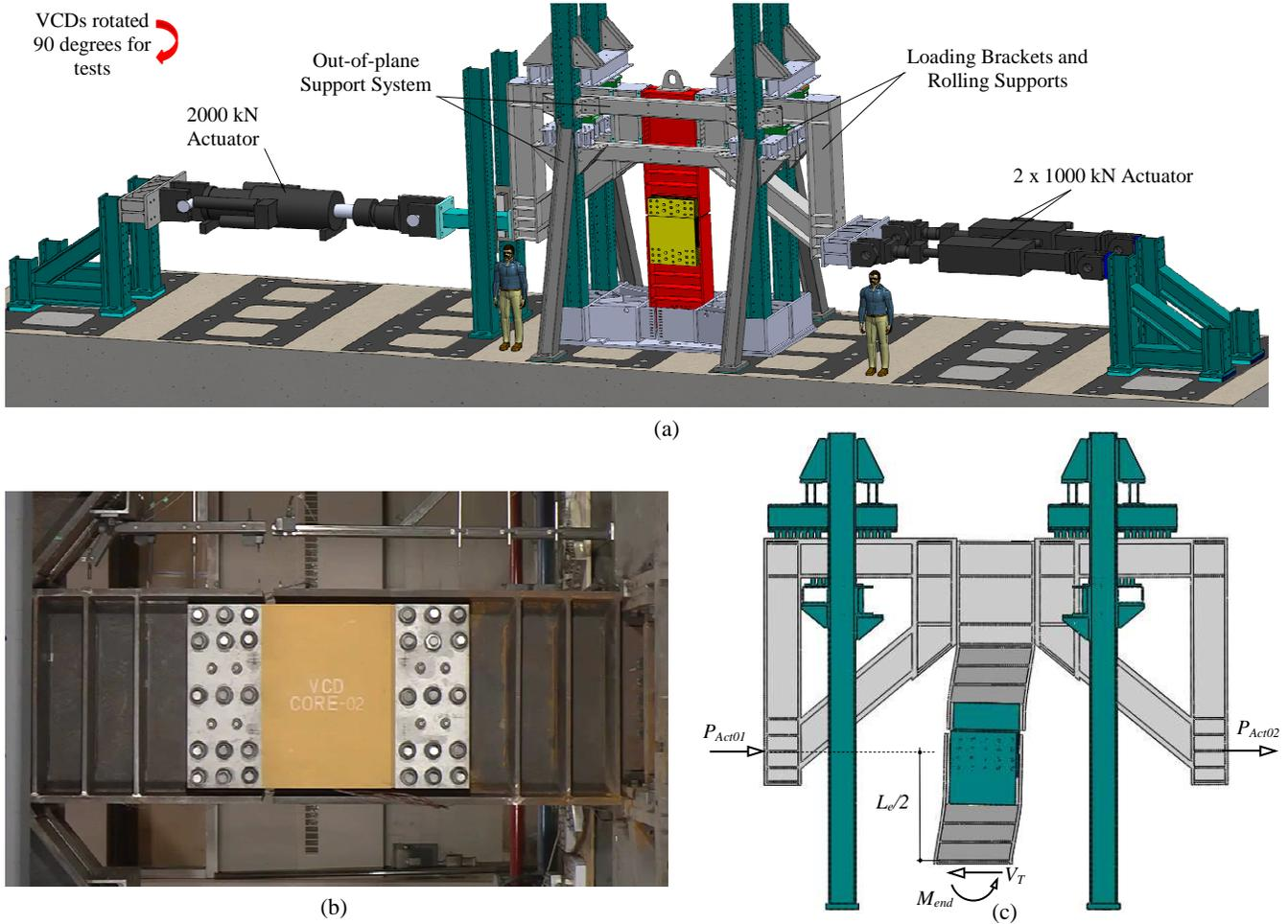
Figure 7. (a) Full scale testing setup (b) Close up rotated photo of VCD specimen (c) Free body diagram
