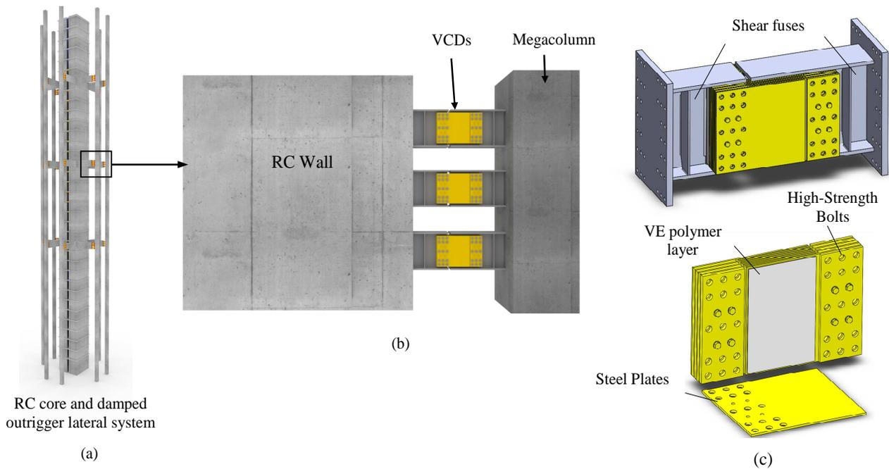
Figure 1. (a) Damped VCD high-rise building, (b) Outrigger detail, (c) VCD and VE panel
