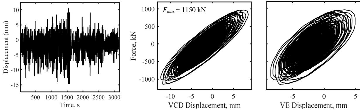
Figure 11. (a) Design level wind testing Protocol (b) VCD hysteresis (c) VE damper panel hysteresis
