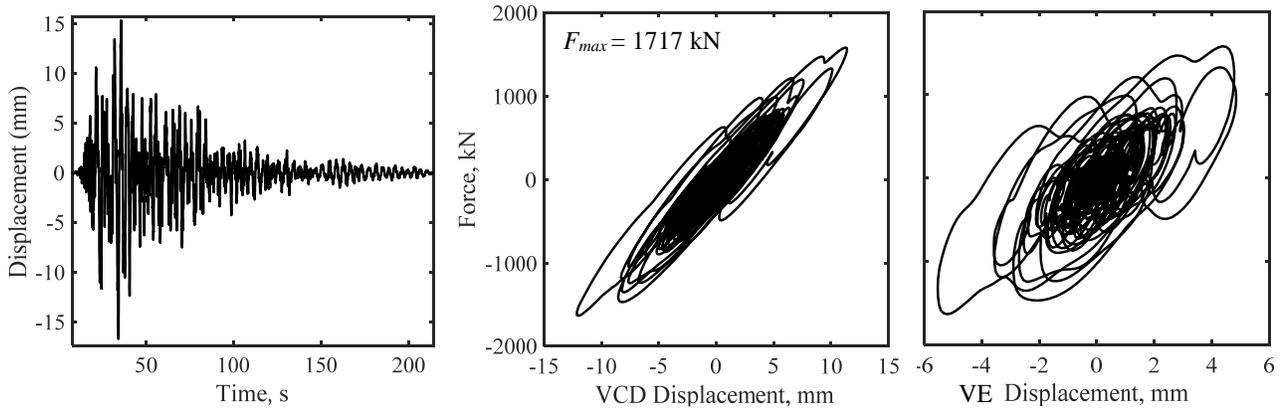
Figure 10. (a) Service level earthquake testing Protocol (b) VCD hysteresis (c) VE damper panel hysteresis
