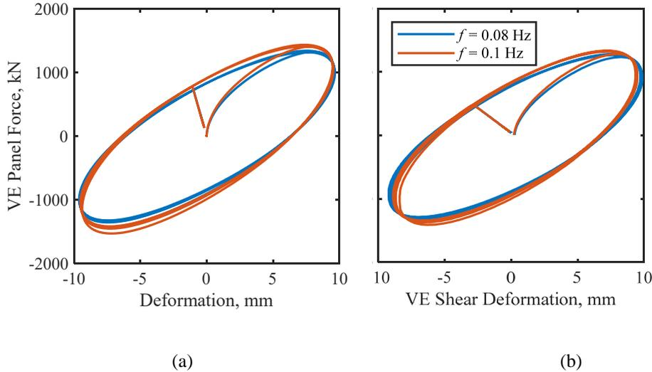
Figure 9. (a) Harmonic hysteresis from MTS test at  $\gamma = 100\%$  and comparison (b) with Full scale shear set up.
