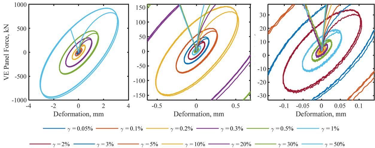
Figure 6. VE Panels A hysteretic response from small to large strains at  $f = 0.3$  Hz.
