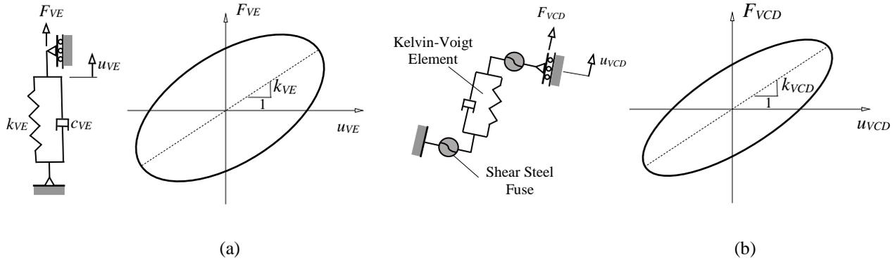
Figure 3. (a) Kelvin Voigt model for VE materials and hysteretic response, (b) Viscoelastic-plastic VCD model and viscoelastic hysteretic response
